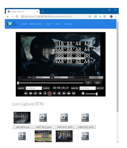
This button brings up a Net-X-Player instance and allows you to select and view any proxy or ABR level live streams being captured using their RTIN files. Clicking on the thumbnails or the name buttons will load the file. The transport buttons can be used to move around the file, and the live button will play at the head of the record.
