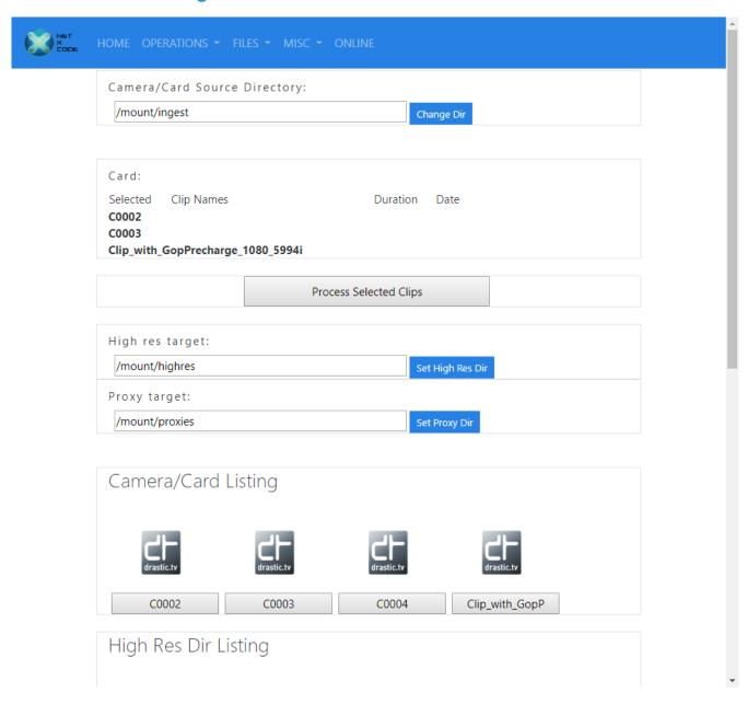
The ingest camera card page allows you to see an incoming camera card, or the directory it was copied to, as a series of recording (clips) rather then the native directory structure of the camera. These clips can be selected and then re wrapped into a single MXF, MP4 or other file, including all stitching for media elements, separate files for tracks and even spanning cards.
