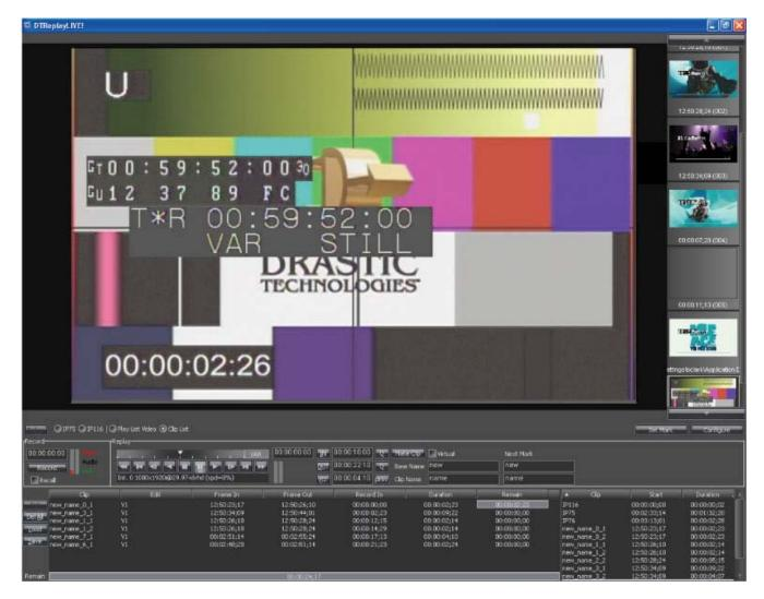
**DTReplayLIVE** is a digital slow motion replay system for SD and HD video signals. It records an incoming video signal in a loop to a local disk array and allows various playback modes for the captured material. **DTReplayLIVE** runs on a multiple channel DDR system. One channel of the DDR is dedicated to VGA display (replay), and at least one separate channel is dedicated to video capture.
