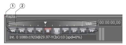
The transport buttons (1) provide (from left to right) Fast Reverse, 5 Seconds Back, 1 Frame Back, Reverse Play, Stop, Pause, Play, 1 Second Forward, 5 Seconds Forward, and Fast Forward.
