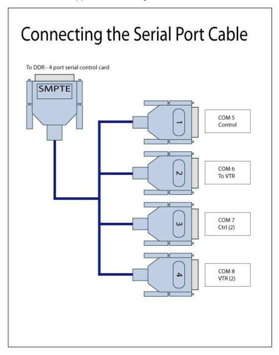
The "To VTR" ports provide control over external VTRs. The "Control" ports provide operation under serial control, as from a controller device or automation system.
