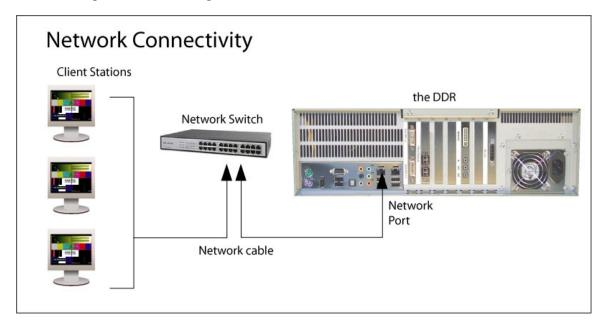
The network port will be situated either in the motherboard connections or as a riser card in the rear of the DDR.
