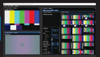
Test Pattern Output to SDI/HDMI, with support for ST-2110 as well as SRT, RTP, UDP, and RIST output.
