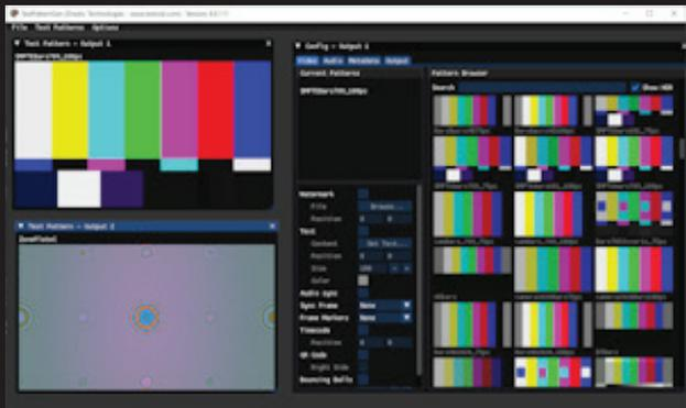
Test Pattern Output to SDI/HDMI, with support for ST-2110 as well as SRT, RTP, UDP, and RIST output.
