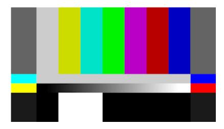
**SMPTE ARIB HD Bars 75%** – SMPTE ARIB HD color bars at 75% saturation.
