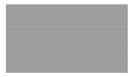
Vertical Pixels One – a series of horizontal one pixel lines for checking vertical resolution
