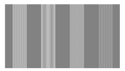
**Horizontal Resolution** – provides a test of horizontal resolution with a series of lines across the screen.
