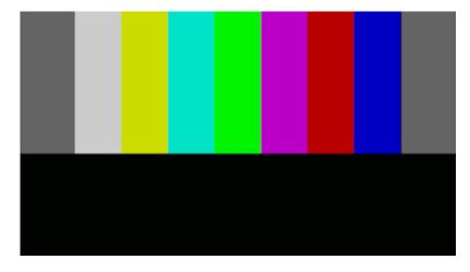
**HD Bars** – features standard HD color bars at 75%, flanked by two gray bars on top, and a panel of black along the bottom.
