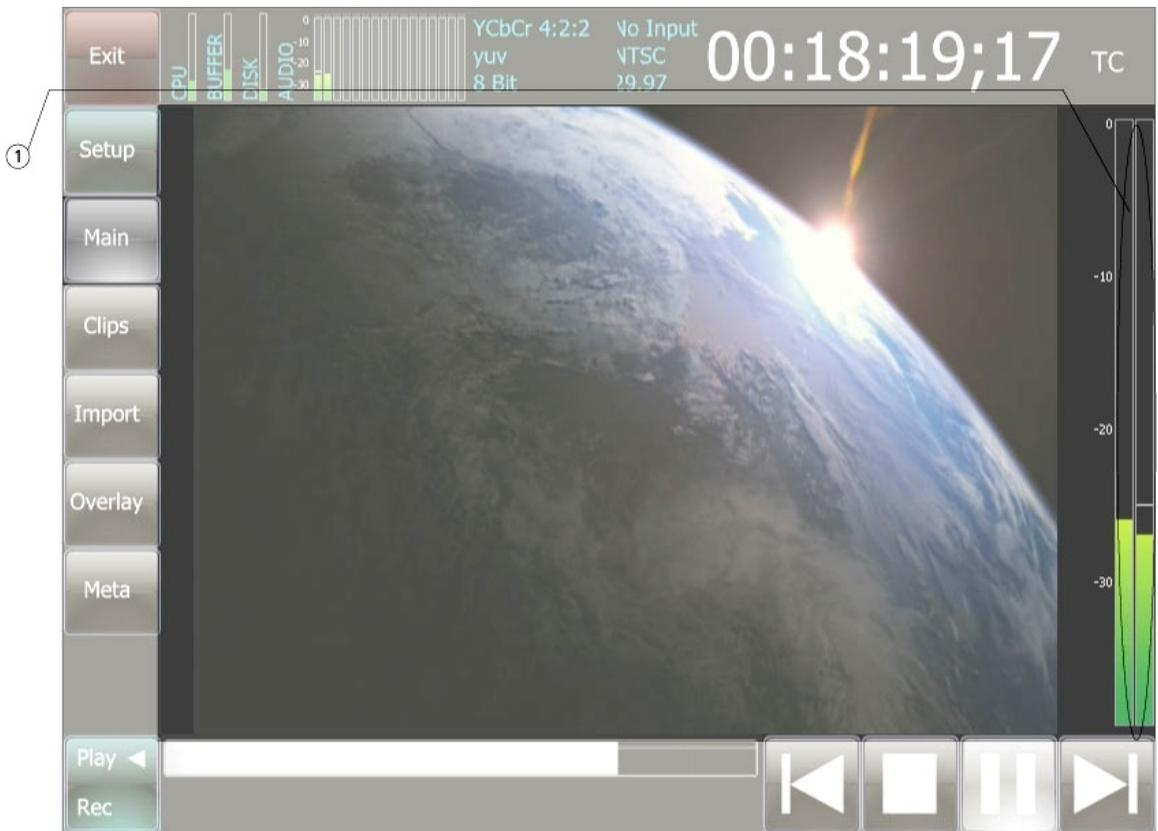
These bars provide a relative signal strength reading for the first audio pair or first two audio channels, to show the user whether their signal is within acceptable parameters for input or output level.
