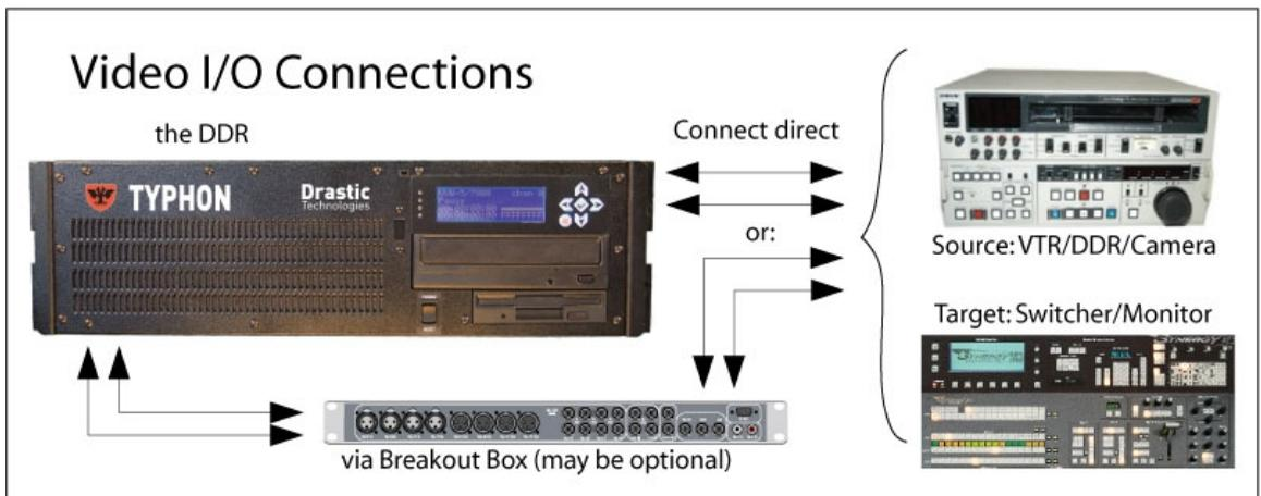
The video input may be confirmed via the video hardware diagnostic, and by viewing a passthrough signal via the onscreen VGA monitor found within each application.
