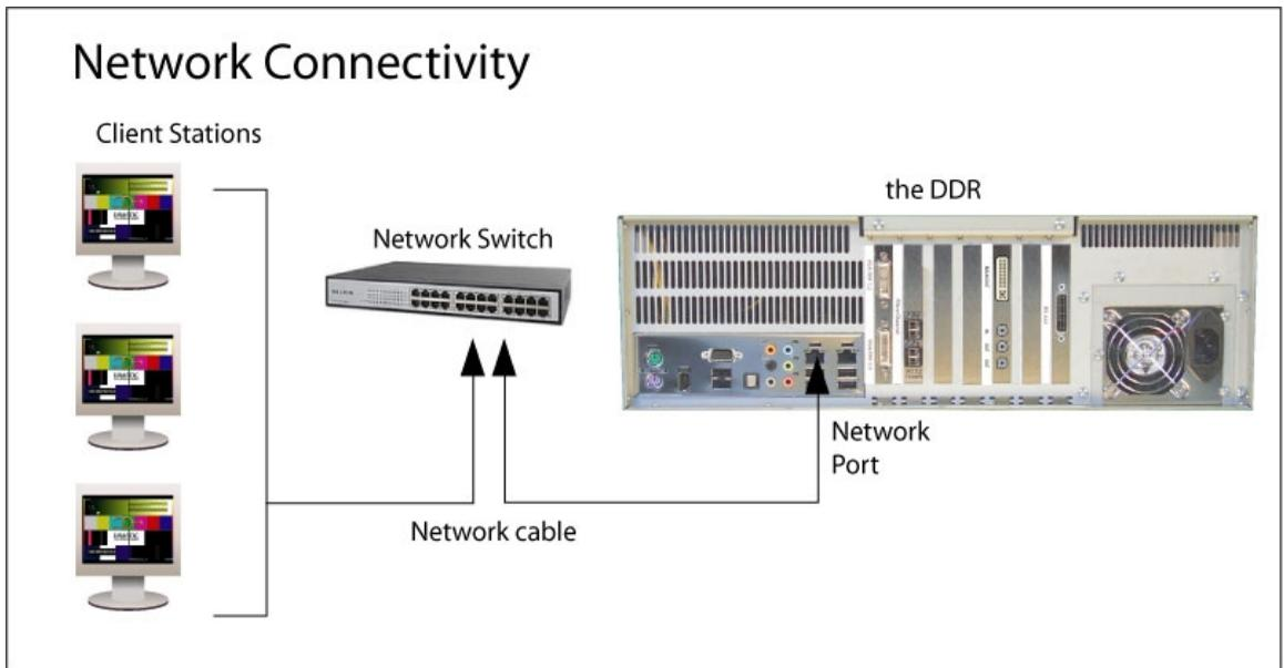
The network port will be situated either in the motherboard connections or as a riser card in the rear of the DDR.
