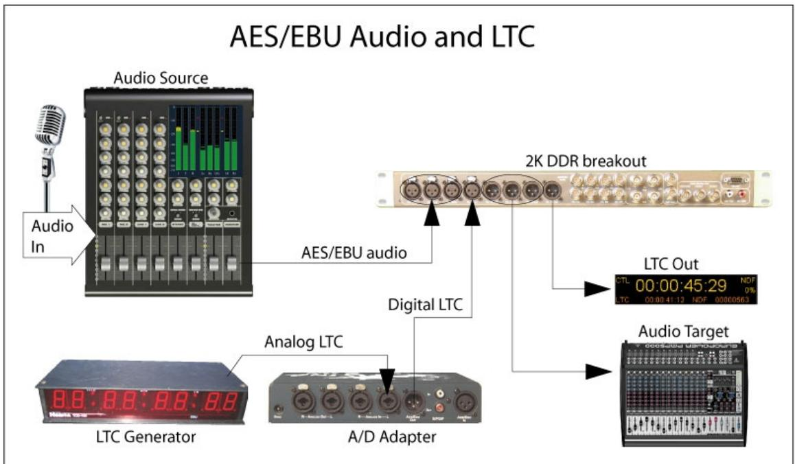
Once the correct connections have been made, each application allows the user to select LTC as the time code source.
