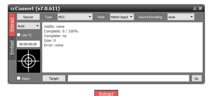
**Extract** button – press to select extract mode – this control turns red upon selection, and causes the interface to display controls specific to the extraction of closed caption files.
