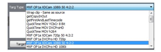
**Targ Type** pulldown menu– the Targ Type pulldown menu allows the user to select a target file type for the file being created during the embedding process.
