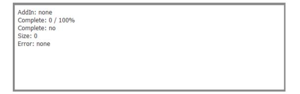
**Summary** field – the Summary field displays details about the add-in (if any), the completion (percentage and yes/no), the size of the created file and whether any errors were observed in the conversion process.
